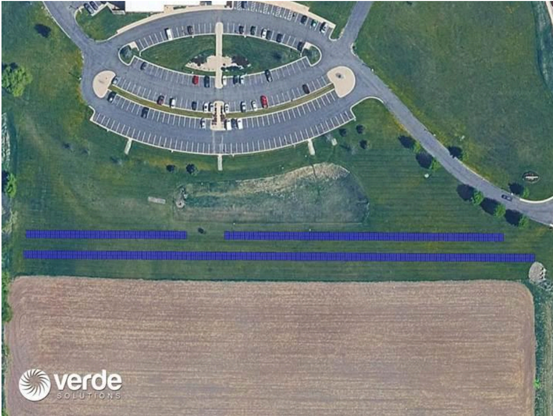
Figure 9: HelioScope design render — proposed ground-mount array south of the Justice Center campus.
