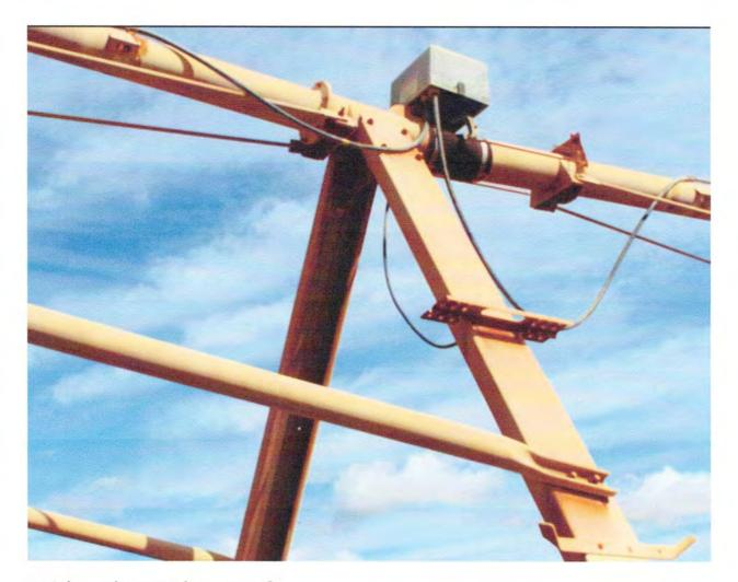
With only 106 hours of pumping the water stripped all the galvanizing off the brand-new center pivot irrigation equipment. This was caused by sulfide s in the Platteville and St Peter being oxidized as acid mine drainage reaction.
