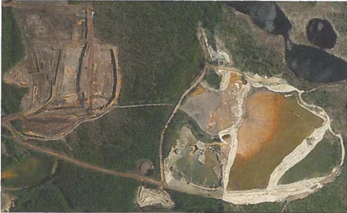
Note. Indicators of AMD in and around a tailings pond at a Minnesota iron ore mine.
