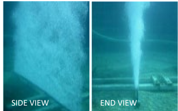
Figure 7. A Bubble Curtain is used in Phase II to consolidate duckweed.
