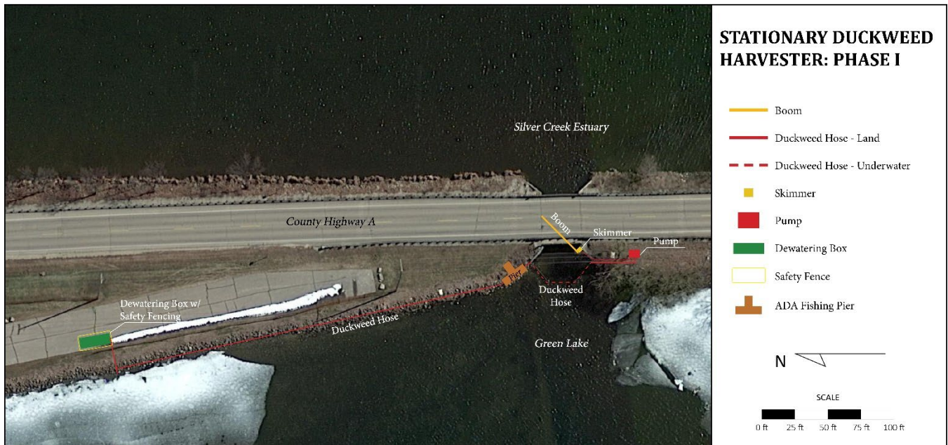
Figure 2. Phase I of the Stationary Harvester will last one week only and utilize a temporary Floating Boom to test the system.
