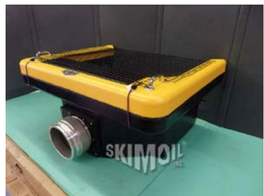
Figure 4. A Skimmer, retrofit with a Bycatch screen discussed later, captures consolidated duckweed.
