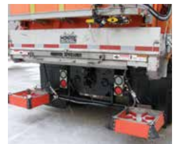
Stationary Bumper Mount Spinners on a One-Way Dual Discharge Spreader
