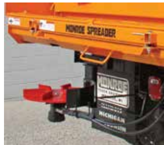
Standard Self Leveling Spinner with Stabilizer Rod
