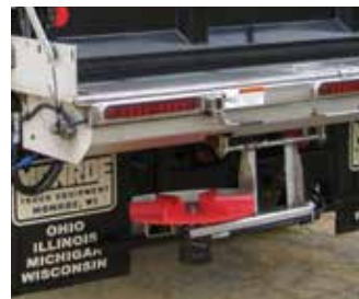
Self Leveling Spinner without Stabilizer Rod
