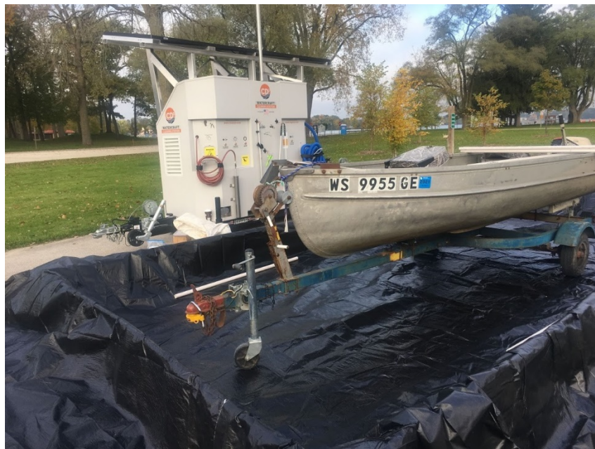
Figure 2. A large tarp was placed on a wood frame to collect small-bodied organisms that were washed off the watercraft in between cleaning treatments.
