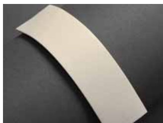
Carlisle Sure-Weld TPO – 60 Weeks (No Failure)
