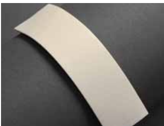
Carlisle Sure-Weld TPO – 60 Weeks (No Failure)
