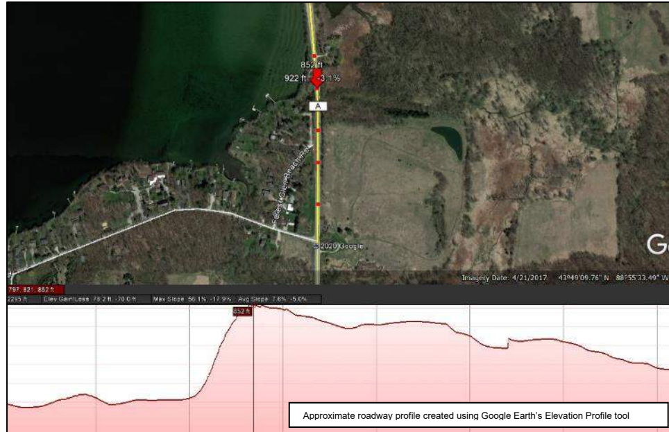
Figure 10 – Approximate Roadway Profile
