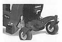
Torsion-Mounted Front Axle Assembly
